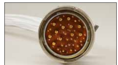
Connectors may contain several different size contacts.
